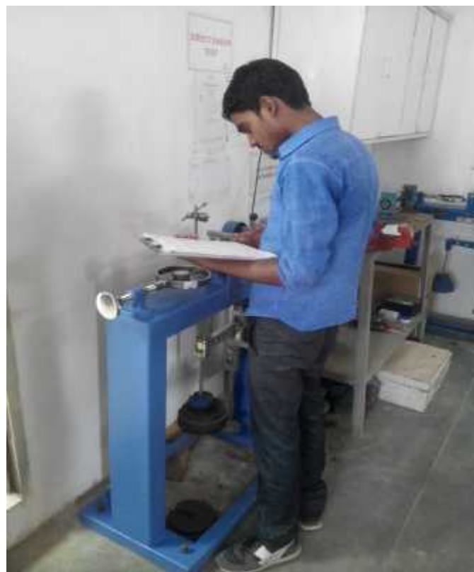
Fig 3.5: Performing Direct Shear
